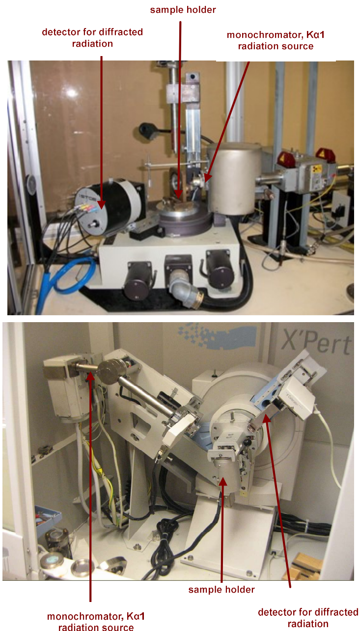
Figure 3.1: Image of the STOE STADI-P (top) and a PANalytical, X'pert PRO powder diffractometer system (bottom) [211].
