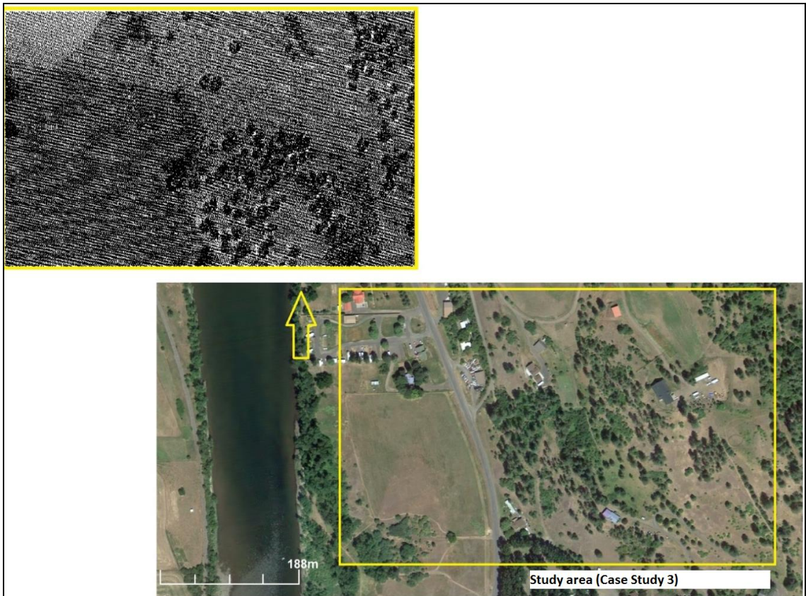
Figure 7-9 Case study 3: Raw LiDAR point data (one million points) and case study area (yellow rectangle on Bing Maps satellite image).
