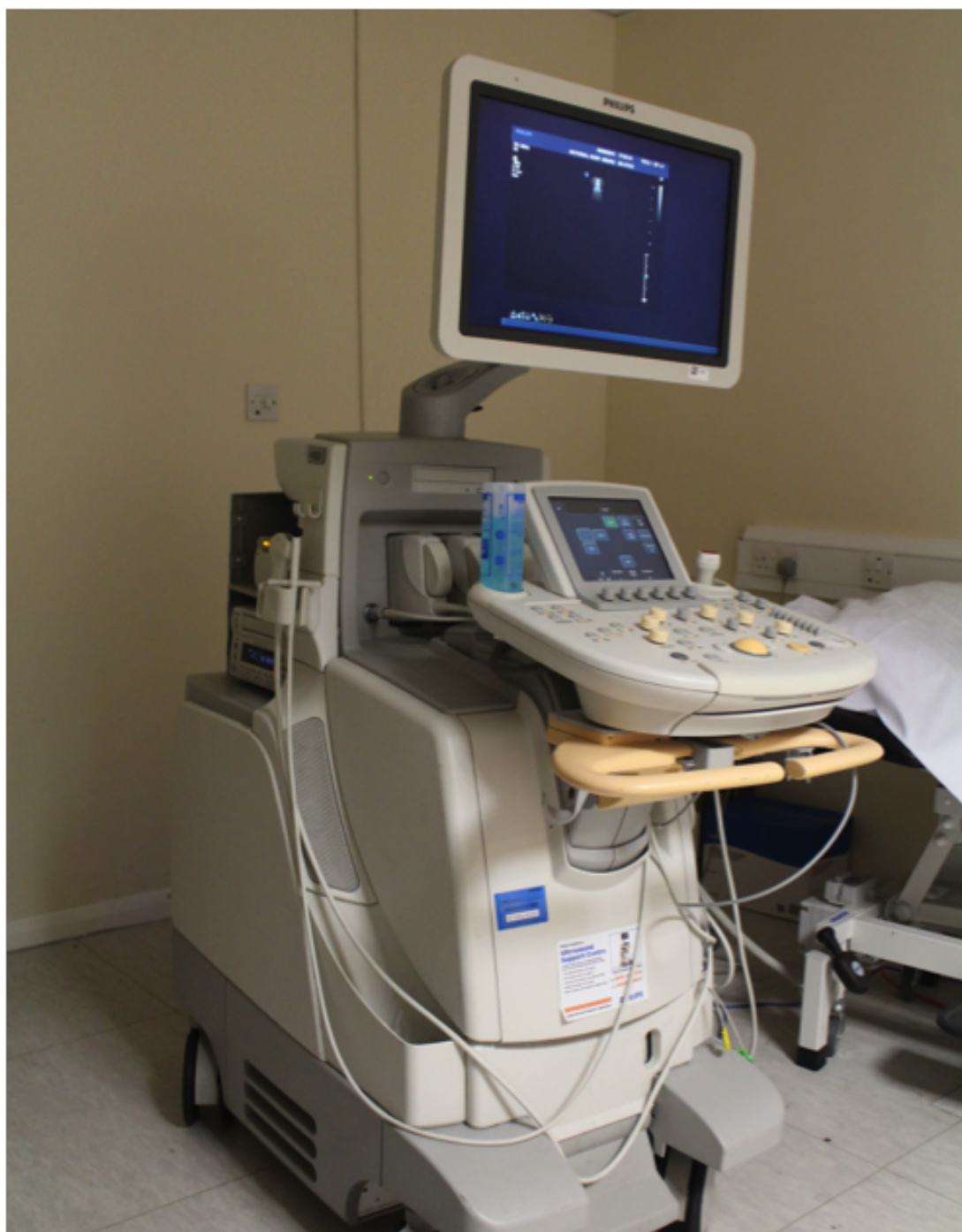
Fig. 7.3: Philips iU22 ultrasound machine with 2.5MHz probe in the Lysholm Department of Neuroradiology at the National Hospital for Neurology and Neurosurgery.
