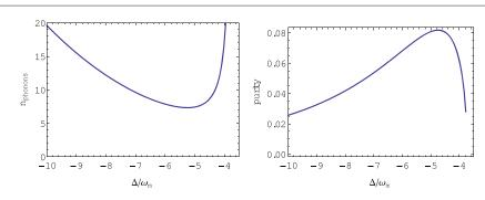
**Figure 2.** Steady-state values for average number of phonons (left) and for the oscillator purity (right), as a function of the detuning  $\Delta$  ( $g = \omega_m$ ,  $\kappa = 2\omega_m$  and  $\Gamma = \omega_m/10$ ). Notice that we plot only values of detuning corresponding to the stable region and that minimum phonon number and maximum purity do not exactly correspond (this is due to the fact that the steady-state corresponds to a squeezed thermal state).
