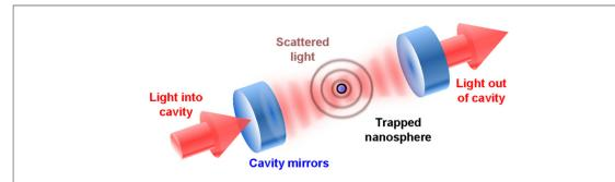
**Figure 7.** Schematic of the experimental set-up for the quantum control of a levitated dielectric nanosphere within an optical cavity. The nanoparticle can be sideband-cooled by sending in light that is red-detuned from the cavity resonance. The light that leaves the cavity can be continuously monitored to perform generaldyne measurements. The light which is scattered by the particle can be collected to give information upon the position of the nanosphere.
