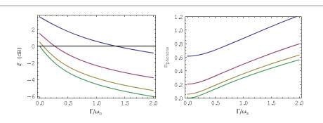
**Figure 5.** Results obtained through analytical calculations for steady-state squeezing in dB scale (left) and number of phonons (right) of a decoupled mechanical oscillator (g = 0) subjected to time-continuous position measurement, as a function of the decoherence parameter  $\Gamma$  and for different values of the measurement efficiency  $\eta_2$ : from top to bottom,  $\eta_2 = \{0.2, 0.5, 0.8, 1\}$ .
