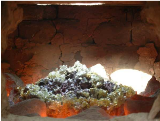
Figure 5.17 Fusing of the batch in the crucible.
