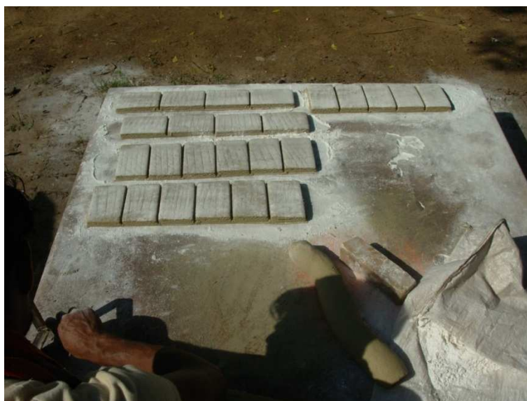
Figure 5.13 Tile bodies being prepared. Note the rolled piece of dough in the shadow in the foreground.
