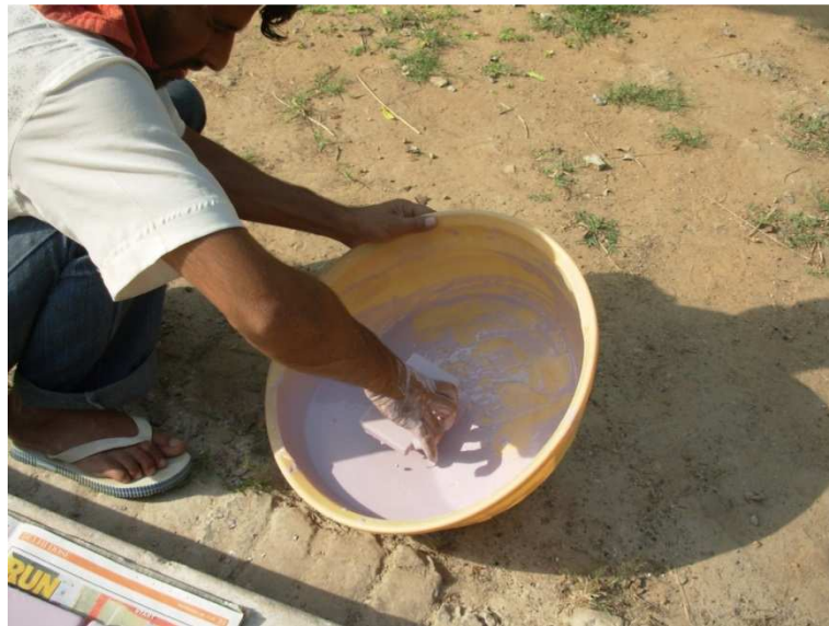
Figure 5.21 A glaze coat being applied on a tile body by dipping it in slurry of the powdered frit.
