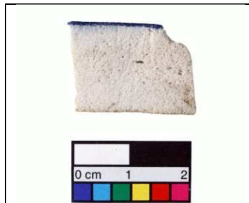
Figure 6.20 Cross-section of a tile sample (SG/02) from Sheesh Gumbad. Note the bright white colour of the body.
