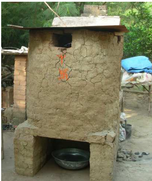
Figure 5.15 A traditional Blue Pottery glaze frit furnace.
