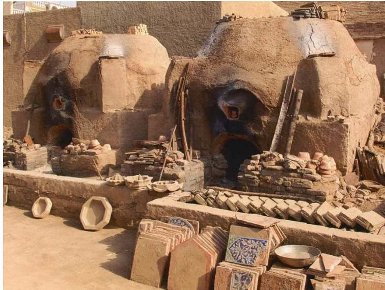
Figure 5.10 A typical kiln employed in the traditional pottery and tile industry in Pakistan. Glass frit to be used for glazing is usually manufactured in-house, mostly utilizing the same kiln (from Akhund and Askari 2011, 66).
