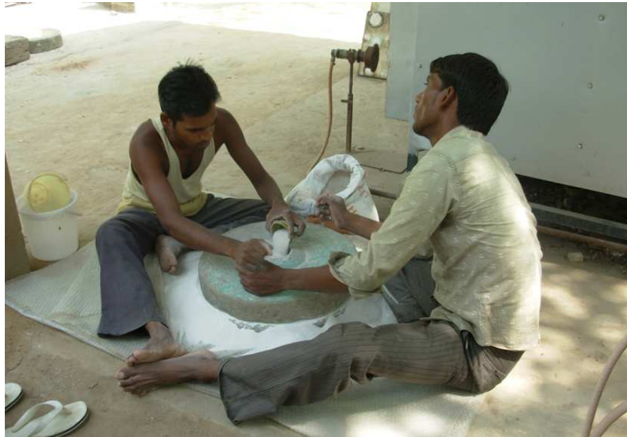
Figure 4.5 Artisans engaged in the crushing of coarse grains of quartz to a fine powder using a traditional stone hand-mill. Live demonstrations of production processes, such as this one, enabled a better appreciation of the technologies involved in the original manufacture of Lodhi and Mughal tiles.
