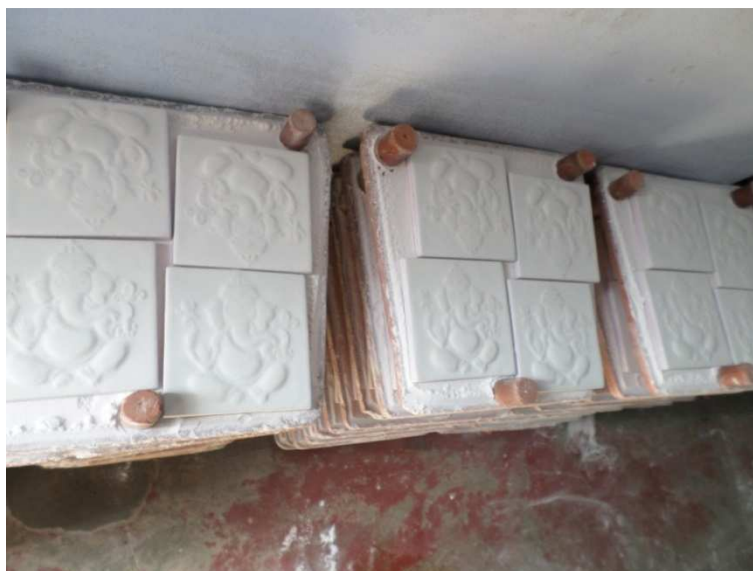
Figure 5.14 A set of relief-embossed tiles coated with an engobe.
