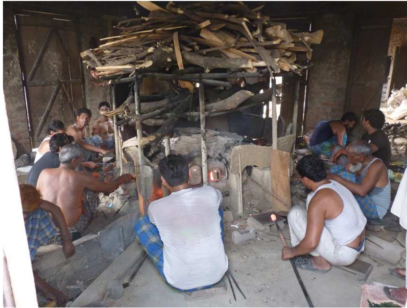
Figure 5.2 A traditional glass-working furnace in operation in Purdalpur. Traditional furnaces for bead and bangle-making, such as this one, still abound in the region. The glass being worked in these furnaces is now sourced from factories at Firozabad.
