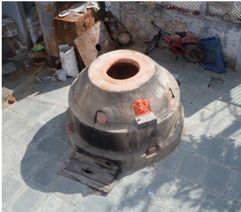
Figure 5.22 A Blue Pottery kiln at the workshop of Anil Jain in Jaipur. The wooden boards on the floor adjacent to the kiln cover the stokehole, the firebox being located beneath the kiln, below ground level.
