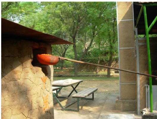
Figure 5.19 The batch being replenished as the frit is formed.
