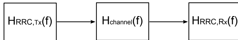
Figure 3.13: Two RRC matching filters are split between the transmitter and receiver, to give an overall RC filter response.
