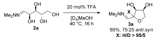
Scheme 4. Postulated mechanism and mechanistic studies.
