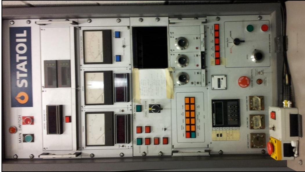
Figure C.17: Engine dynamometer speed, and oil and coolant level and temperature control unit
