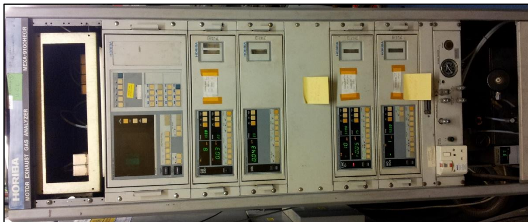
Figure C.15: Exhaust gas emissions analyser rack (Horiba MEXA-9100HEGR)
