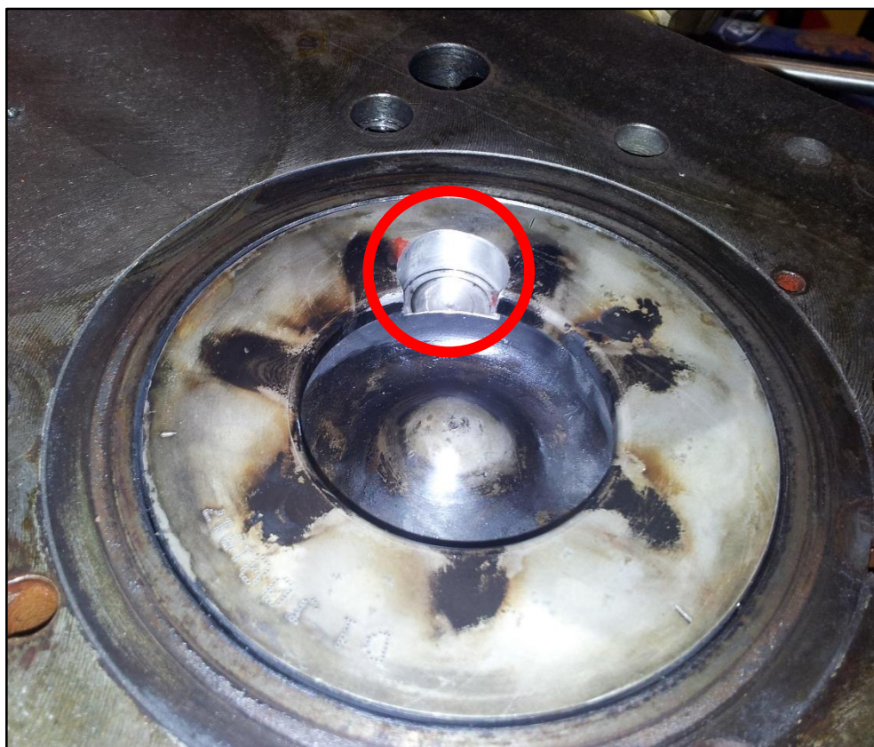
Figure C.3: A small part at the edge of the piston bowl (of diameter 15 mm and depth 10 mm) was removed to prevent the sampling valve tip from hitting the piston
