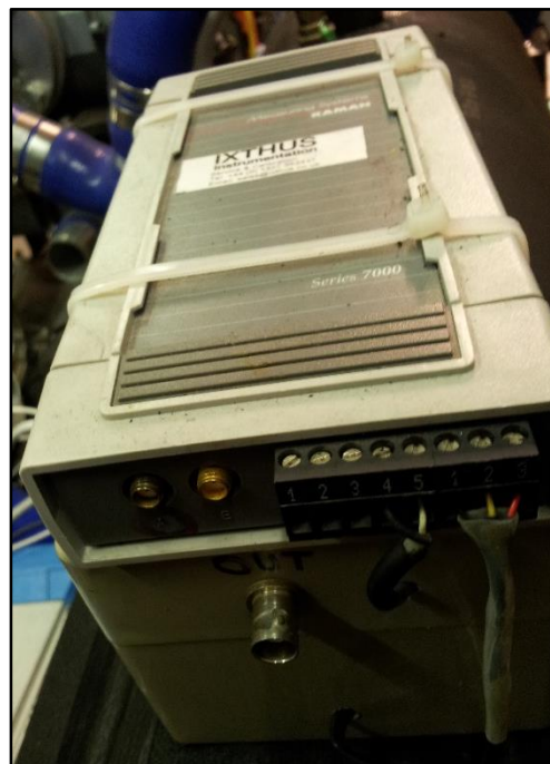
Figure C.6: The amplifier electronics box and power supply for the LVDT proximity sensor mounted on the gas sampling valve
