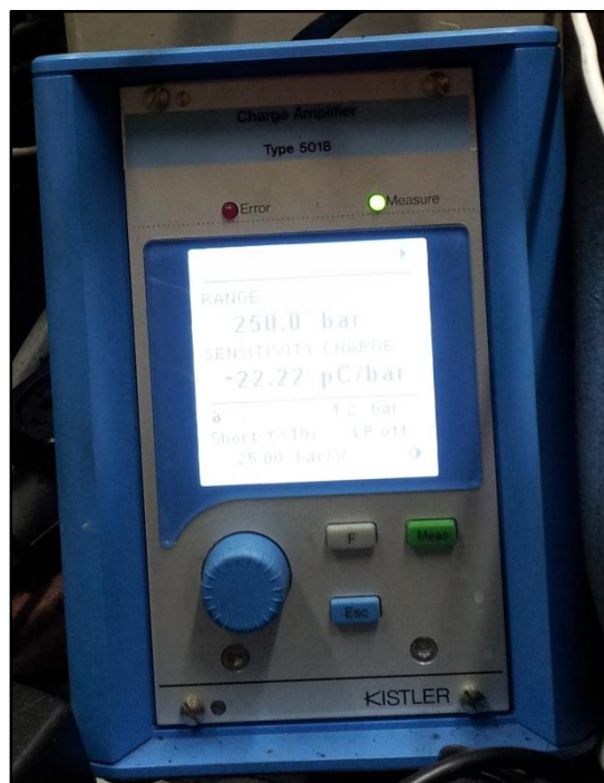
Figure C.8: Kistler charge amplifier (type 5018) for use in conjunction with the piezoelectric transducer mounted on the engine head to measure in-cylinder gas pressure
