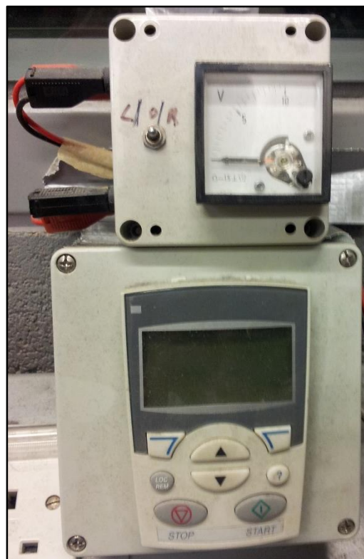
Figure C.12: Potentiometer controller to control the speed of the electric motor, which drives the supercharger in the intake air boost system
