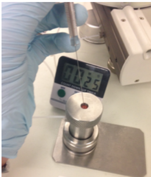
Figure A.6: Operation of the liquid/gas injection port, installed onto the EA-IRMS.
