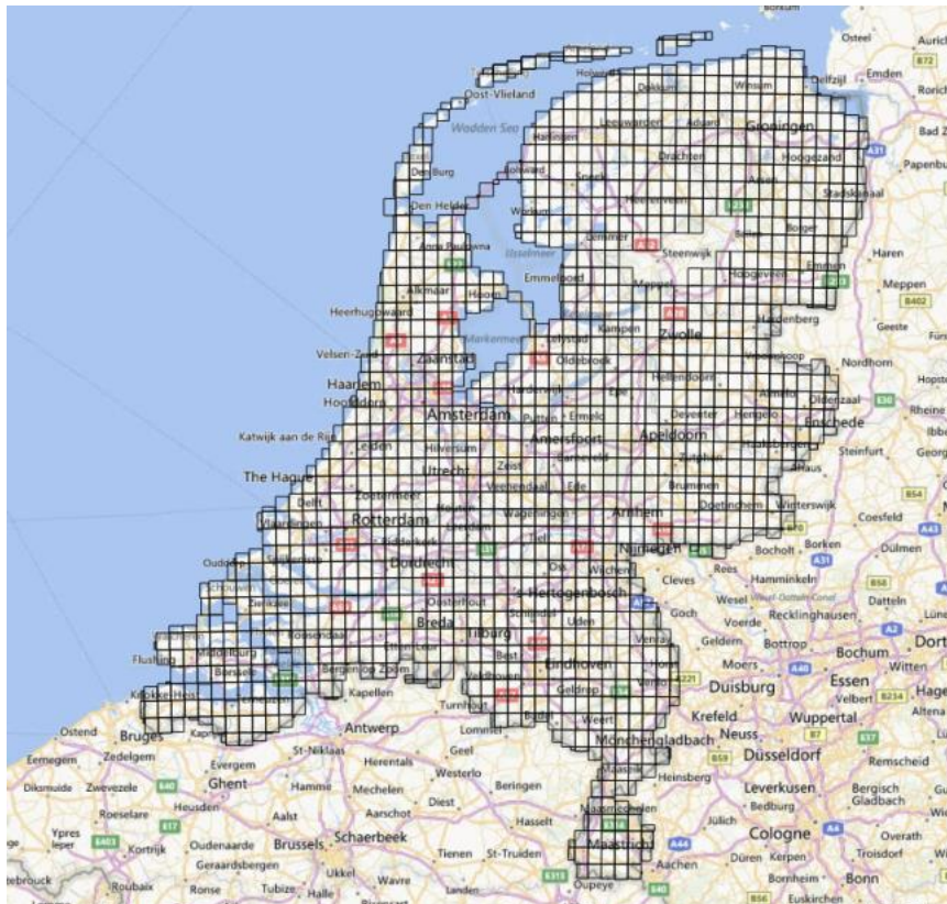
Figure 4: Bounding Polygons of the tiles of the AHN2 dataset displayed over a map.
