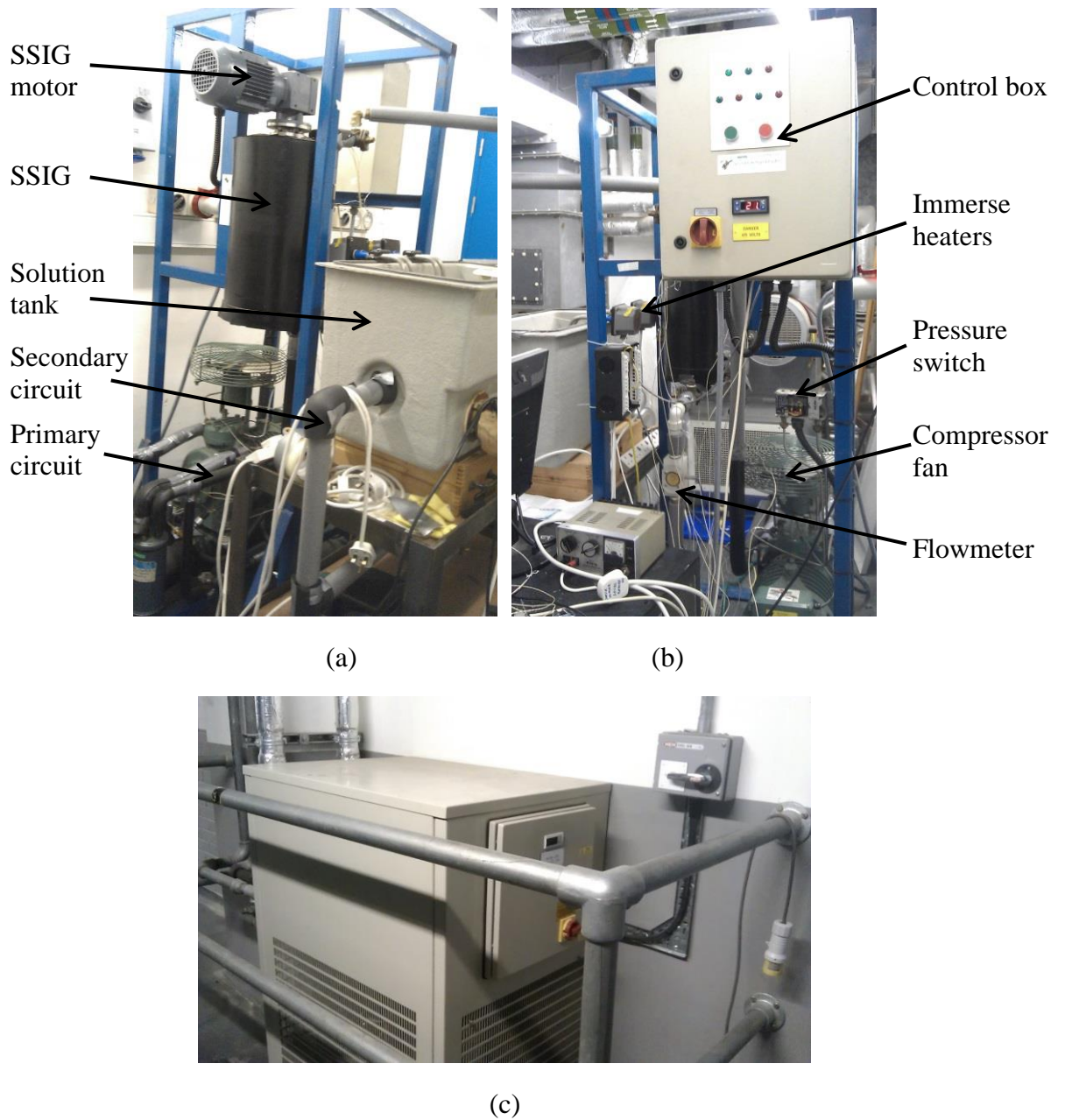
Figure 3.1 Test rig, (a) and (b): primary and secondary circuit, (c): chiller unit for the condenser cooling water.
