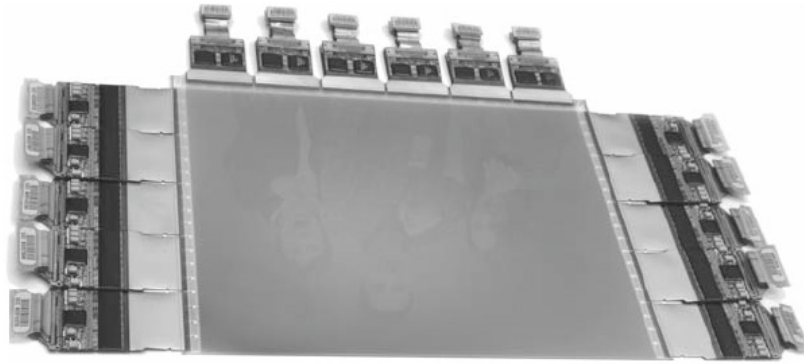
Figure 2.2. Photo of flat-panel detector. (Courtesy, GE Global Research Centre)
