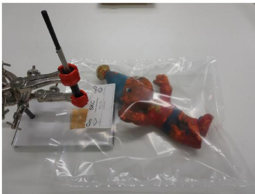
Figure 7. Non-destructive analysis of a PUR foam doll using a SPME fibre in a manual holder (should be in colour in printed version)
