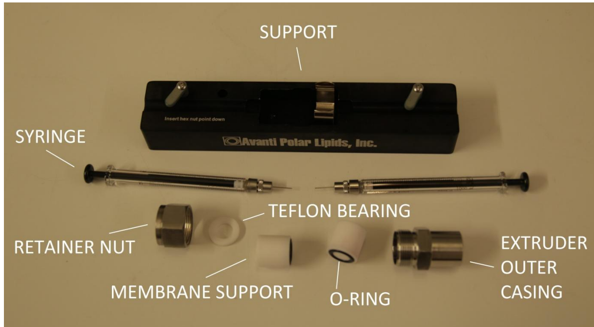
Figure 5.1 Liposome extruder and support with 1 mL air tight glass syringes (Avanti Polar Lipids). A polycarbonate membrane flanked by filter supports is placed between two teflon membrane supports and the system is locked using an outer casing and a nut. The extruder containing the membrane is then placed on a support and the syringes are introduced into the membrane supports through the sides.
