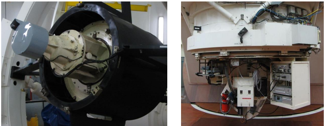
Figure 3.12: Swapping the Wide-Field Camera for the secondary mirror (left). Intermediate Dispersion Spectrograph (right)
