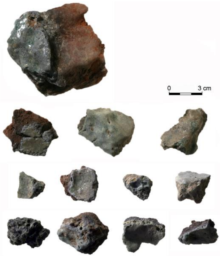
Fig. 3. Fragmentary glazed (vitrified) and unglazed fired mud-bricks from workshop furnace.
