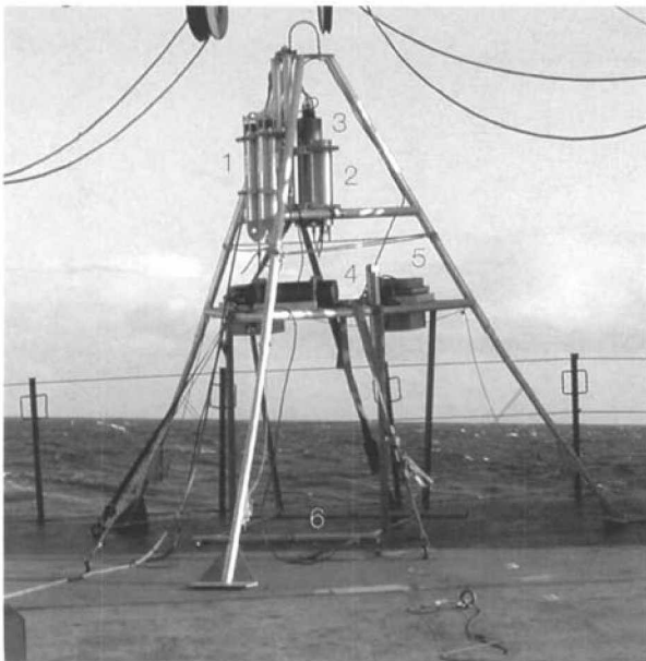
Fig 6: The 'Sprint' Lander. (1) Acoustic releases, (2) High speed camera, (3) Controller, (4) Electric stimulator, (5) Battery, (6) Electrode array
