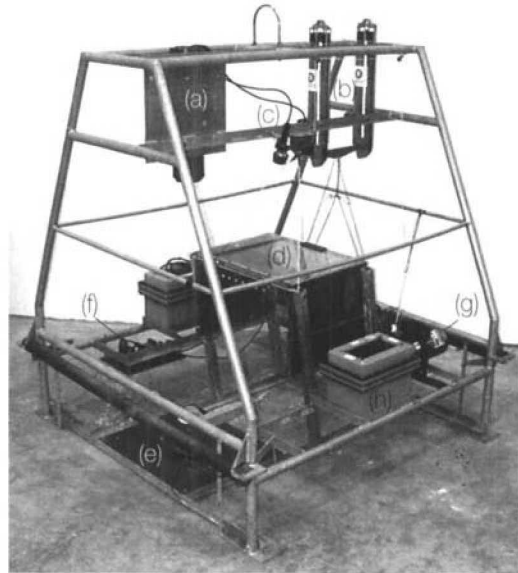
Fig 9: The FRESP Respirometry Lander; (a) Internally recording digital video camera; (b) acoustic releases; (c) Lights; (d) respirometry chamber in its raised position; (e) respirometry chamber base plate (bait located in the centre of the plate); (f) oxygen sensor and pump; (g) controller and data logging; (h) battery
