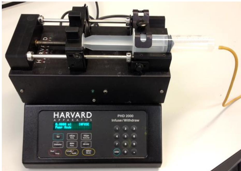
Figure 2.18: The syringe pump used to pass water through a flow phantom within the bore of the MRI scanner.
