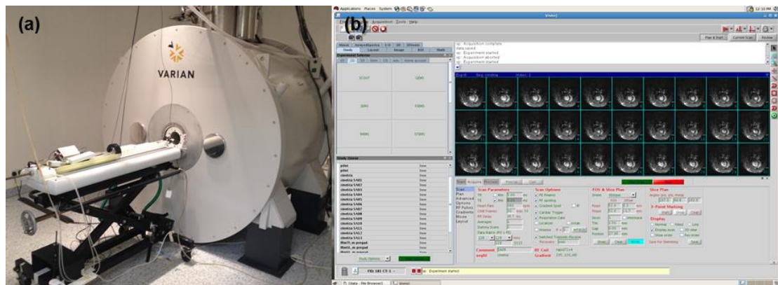
Figure 2.14: (a) The Agilent 9.4T scanner in CABI and (b) a screenshot of the software, VNMRJ, used to control the scanner.
