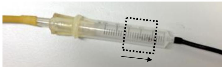
Figure 3.5: Photograph of the custom-built flow phantom. The phantom was constructed using a 5ml syringe. Water was driven (in the direction of the black arrow) by a syringe pump via rubber tubing through the phantom and into a water reservoir at the rear of the MRI scanner. The dotted line represents the approximate location of the imaging slice.
