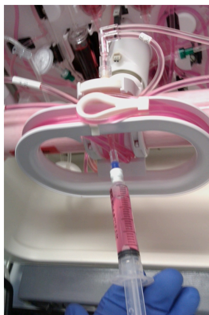
Figure 2.3: Taking sterile media samples from the bioreactor. Samples are drawn from the IC loop through a 0.22 \mu m filter into a Luer Lock syringe.
