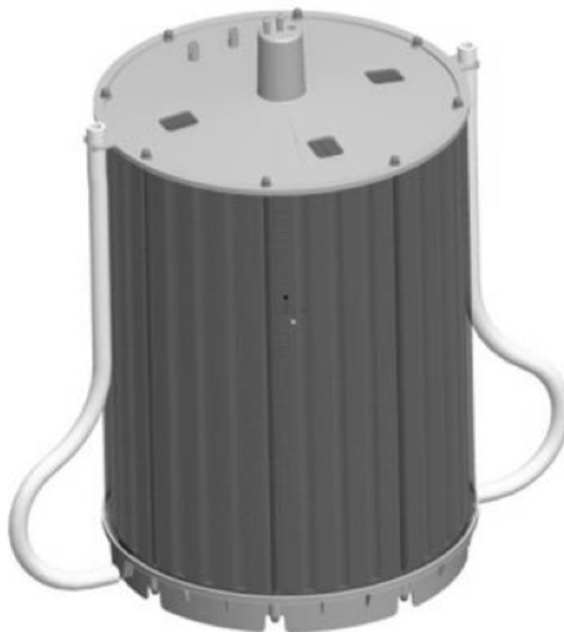
Figure 3.1: Overview of the Integrity Xpansion Multiplate bioreactor (Pall). a) The Xpansion system with its control unit. b) A computer model of the multilayer system within the reactor b)
