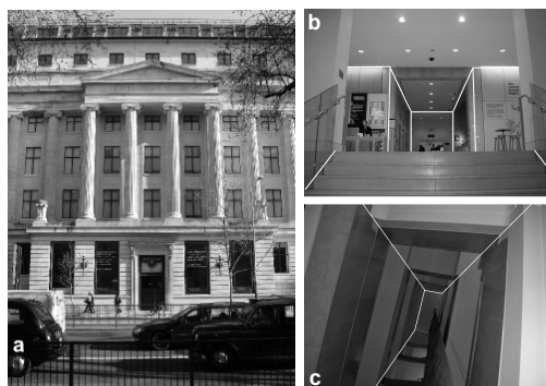
Figure 5.1: The Wellcome Collection building. (a) façade of the building, (b) main hall, (c) staircase. The lines overlapped in images (b) and (c) indicate the shape of the computational geometry that we will use for the simulations.
