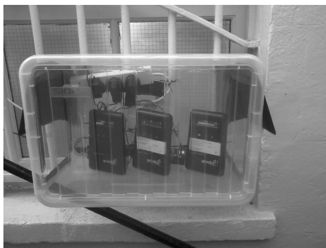
Figure 8.6: Protective case used to cover the particle counting instruments during extended monitoring periods.
