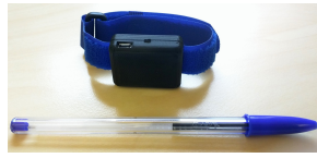
(a) Electronics front and back view. Scale in centimeters. (b) Prototype enclosed in 3D printed box attached to wristband.
