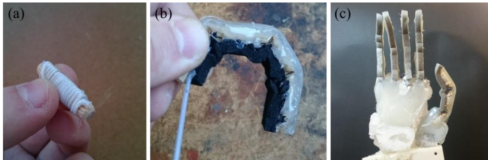
Figure 4. In this design, links are made of wood which carry the pulleys that allow the translation of actuator force through the fingers (a). Wood links are connected to each other with soft HMA material to form soft joints and contribute to the overall flexibility of the manipulator. Finger pads are covered with soft sponge materials to assist form closure (b). By repeating the same finger design, a hybrid manipulator that resembles the human hand is created. Palm is reinforced with rigid materials for the fingers to apply necessary forces during grasping (c).
