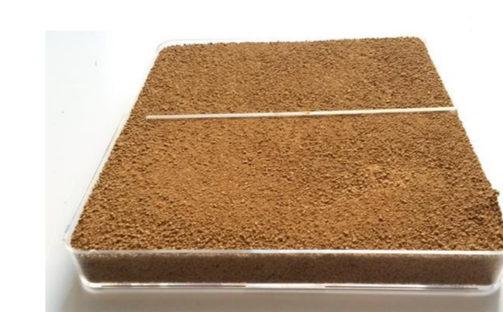
Figure 3 : Design of soil filled rhizotron for analysing Fe-P/ Al-P accessibility in subsoil by wheat plants
