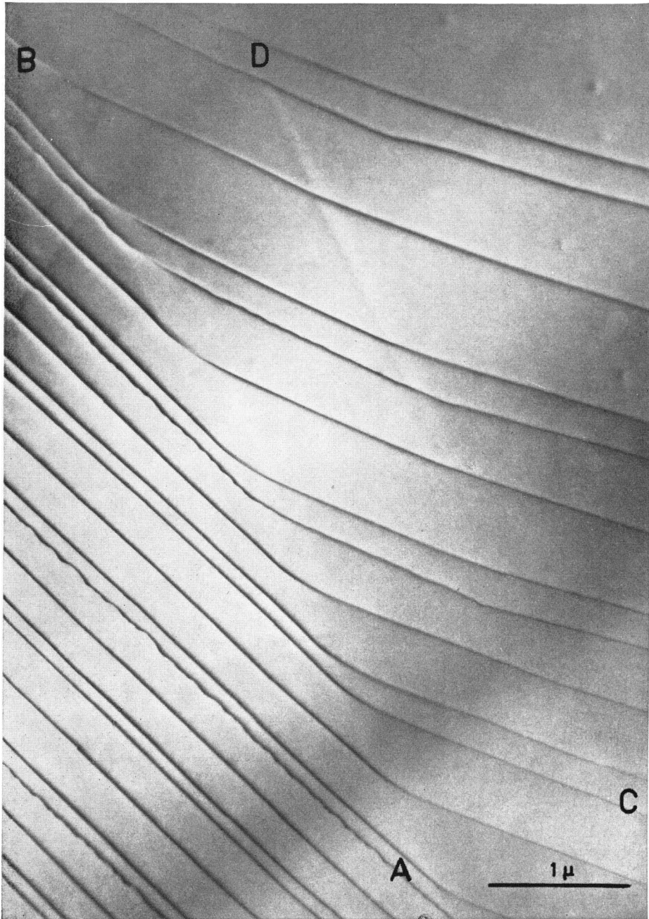
Fig. 15. "Refraction" of a family of ribbon and of unextended dislocations by two sequences of steps AB and CD. On refraction the ribbon width changes as well
