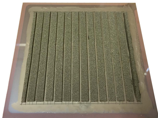
Figure 8 | Photograph of a large-scale photovoltaic water-splitting device. The total device area was 64\text{ cm}^2 with an active area of 52.8\text{ cm}^2 . Each base unit consists of two series-connected a-Si:H/ \mu\text{c-Si:H} tandem solar cells with a cell stripe width and length of 2.5 and 80 mm, respectively. Thirteen base units were neighbouring on a 10 \times 10\text{ cm}^2 substrate. The back end was made of laser-cut nickel-foam elements for both cathodes and anodes. A photograph from the front side of a similar device can be found in Supplementary Fig. 9.
