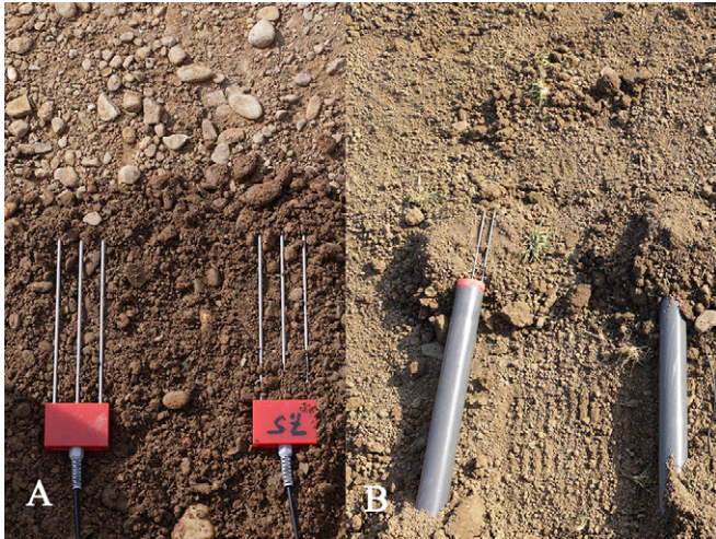
Fig. 5. Time-domain reflectometry (TDR) sensors in the (A) upper and (B) lower facilities. The bases of the TDR sensors were refitted to a round shape attached to a plastic pipe for inserting into the bored holes in the lower facility.
