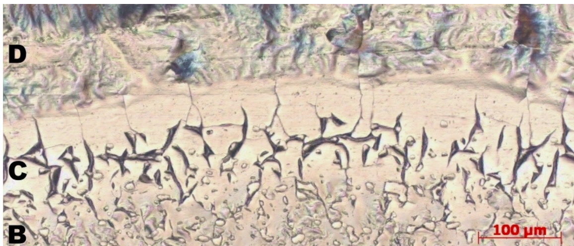
Figure 3.13.: Magnification of laser spot border of figure 3.12a (optical bright field microscopy). The letters indicate the same regions as in figure 3.12f.
