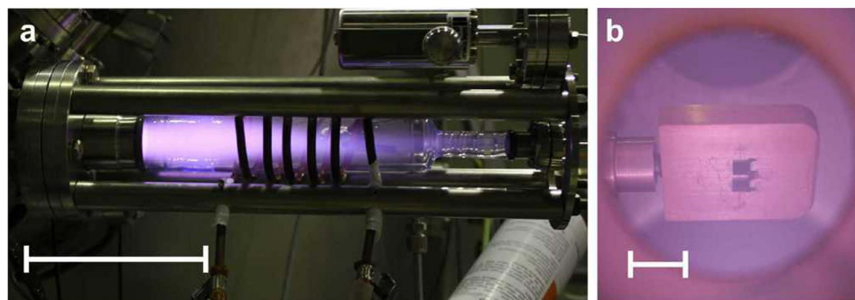
Figure 1. Hydrogen plasma. (a) Photograph of the plasma chamber with ignited hydrogen plasma at UE46-PGM1, HZB-BESSYII. Scale bar is 10 cm. (b) Photograph of two samples on a sample holder in the hydrogen plasma region. Scale bar is 1 cm. The samples are facing to the glass part of the plasma chamber, the photograph was taken through a window above.
