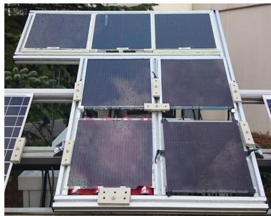
Figure 1: Photographs of solar modules on thermal insulating building materials (left) and the modules under consideration on the outdoor measurement setup (right).
