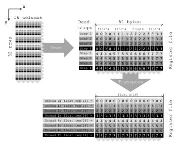
FIGURE 3.9: Local transpose with registers.
