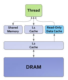
FIGURE 1.7: Kepler and Fermi memory hierarchy according to [22]. The general purpose read-only data cache is known on Fermi architectures as texture cache, as historically it was only used to read textures from global memory.
