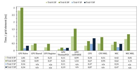
FIGURE 3.13: Grid element execution times per grid element on a  $240 \times 256 \times 256$  cube domain. X dimension is chosen to be 240 to alleviate the effect of caching and algorithmic inefficiencies which occurs on sizes of power of 2 as it can be seen on Figures 3.10,3.11,3.12. Missing bars and n/a values are due to non-feasible or non-advantagous implementations in the Y dimension.
