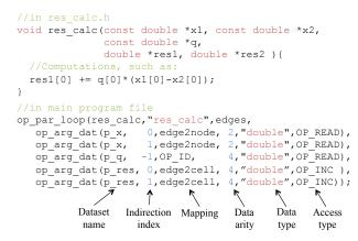
FIGURE 7.1: Demonstrative example of the OP2 API in Airfoil: parallel execution of the res\_calc kernel function by the op\_par\_loop for each elements in the edges set.
