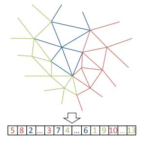
FIGURE 7.2: Demonstrative example of block coloring: edges are partitioned into three blocks colors. Indices of edges belonging to different colors are shuffled in the linear memory.
