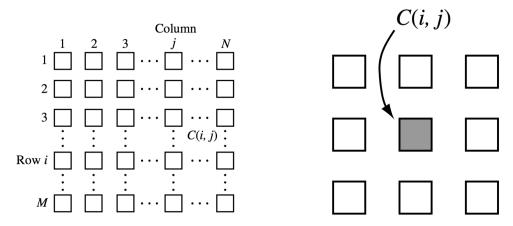
FIGURE 6.1: Left: standard CNN (Cellular Neural Network) architecture. Right: CNN local connectivity to neighbor cells. Source: [64]
