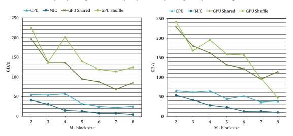
FIGURE 4.5: Single (left) and double (right) precision effective bandwidth when solving block tridiagonal systems with varying M block sizes. Bandwidth is computed based on the amount of data to be transfered. Caching in L1 and registers can make this figure higher then the achievable bandwidth with a bandwidth test.
