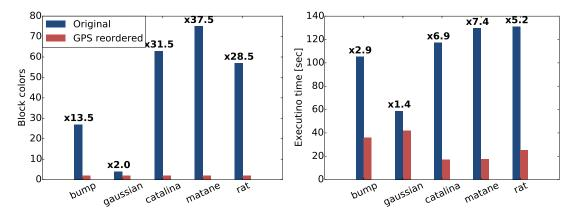
(A) The effect of mesh reordering on the block (B) The effect of mesh reordering on the execolors is significant.
