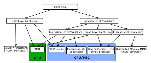
FIGURE 1.1: Classification of parallelism along with parallel computer and processor architectures that implement them.
