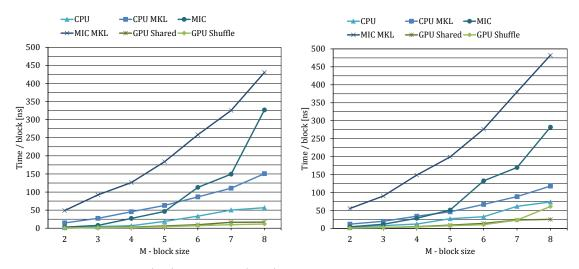
FIGURE 4.7: Single (left) and double (right) precision block-tridiagonal solver execution time per block matrix row for varying block sizes.
