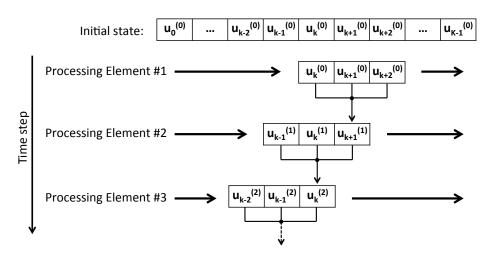
FIGURE 5.1: Stacked FPGA processing elements to pipeline stencil operations in a systolic fashion. The initial system variables  $u_0^{(0)}, ..., u_{K-1}^{(0)}$  are swept by the first processing element. The result  $u_{k+1}^{(1)}$  is fed into the second processing element.
