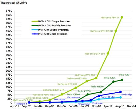
Apr-01 Sep-02 Jan-04 May-05 Oct-06 Feb-08 Jul-09 Nov-10 Apr-12 Aug-13 Dec-14 FIGURE 1.5: The increase in computation power. A comparison of NVIDIA GPUs and Intel
