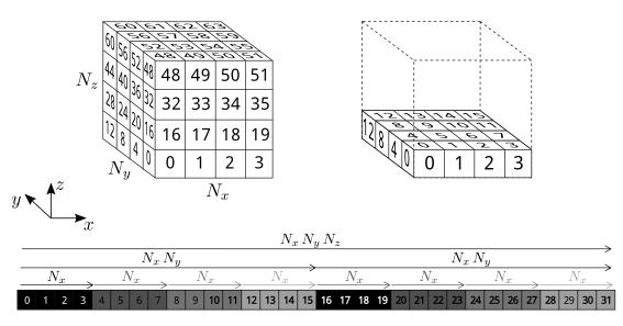
FIGURE 3.4: Data layout of 3D cube data-structure.
