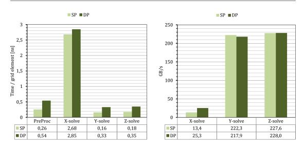
FIGURE 3.7: ADI kernel execution times on K40m GPU, and corresponding bandwidth figures for X, Y and Z dimensional solves based on the Thomas algorithm. Single precision Xdimensional solve is slower  $\times 16.75$  than the Y dimensional solve. Bandwidth is calculated from the amount of data that supposed to loaded and stored and the elapsed time. High bandwidth in the case of Y and Z dimensional solve is reached due to local memory caching and read-only (texture) caching.
