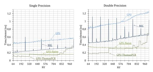
FIGURE 3.12: Single and double precision execution time per grid element. 65536 tridiagonal systems with varying NY length along the Y dimension are solved. CPU, MIC and GPU execution times along with the comparison of the best solver on all three architectures are show.
