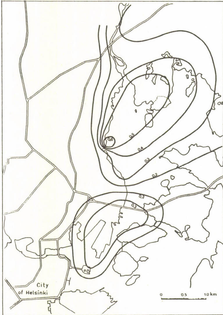
Fig. 3. Mean monthly accumulation of cadmium (ppm dry weight) in moss-bags in Helsinki during the winter of 1982/1983. Interpolated graphs of equal value are shown.
