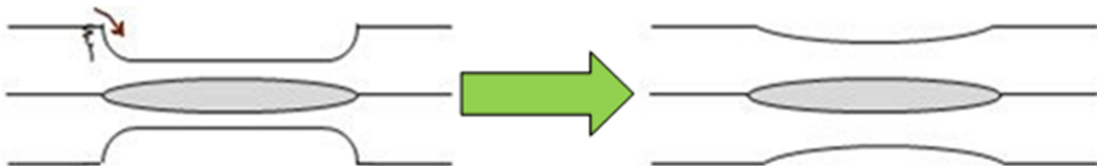
Figure 6. Influence of different radii of electrode caps (schematic).
