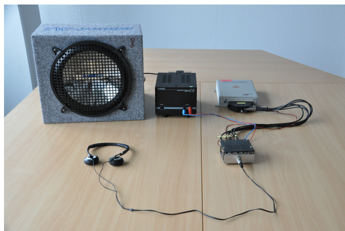
Figure 5.3: Schematic representation (top) and photograph (bottom) of the experimental setup for the ANC system
