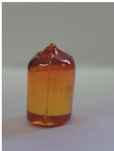
Figure 2 The Ru-doped \text{LiNbO}_3 single crystal grown along [001].
