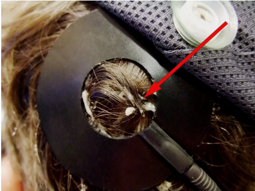
Figure 4. Example of leaking EEG gel creating direct contact between tACS and EEG electrodes. Leaking EEG gel, which creates direct contact between the tACS and the EEG electrode, is observed. Bridging such as this between the tACS and EEG electrodes can be created e.g., by adding an excess amounts of EEG gel under the tACS electrode or the EEG electrode in the vicinity of the tACS electrode, or by the tACS electrode being moved. Please click here to view a larger version of this figure.
