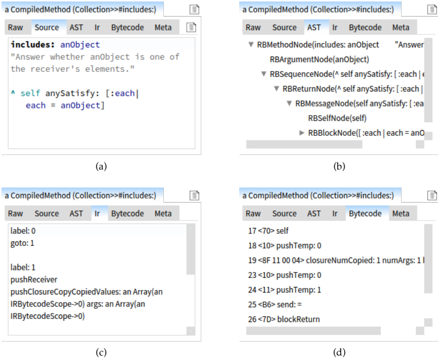
Figure 4.8: Domain-specific views for CompiledMethod objects: (a) Source code; (b) Abstract syntax tree; (c) Intermediate representation; (d) Bytecode.
