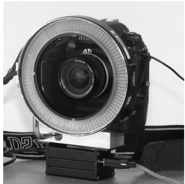
Figure 5. Mounting of the ringflash to the camera's tripod mount to relieve the filter thread of the lens off the extra load.
