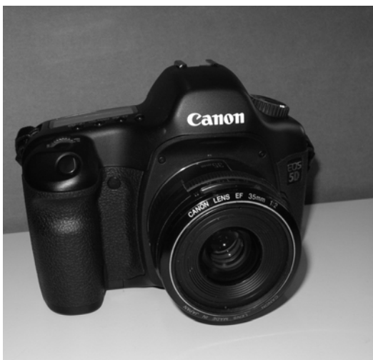
Figure 1. Canon EOS 5D with EF 2/35 mm lens where the focusing tube was fixed with epoxy (indicated by the whitish ring around the focusing tube).
