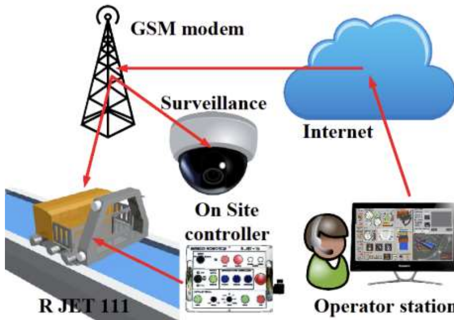
Figure 4 Modbus based TCP/IP communication network for the remote control and supervision of R JET 111
