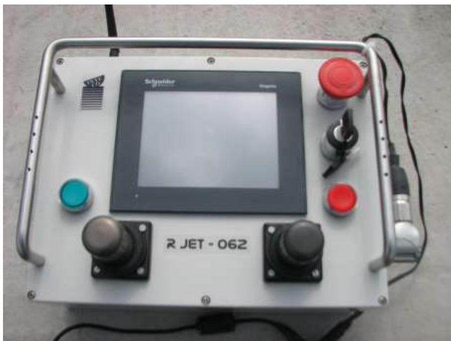
Figure 3. Remote control console for operating a robot from safe distance.
