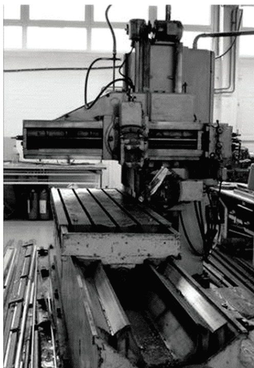
Figure 3 Planning machine used as a base for experimental machine tool development
