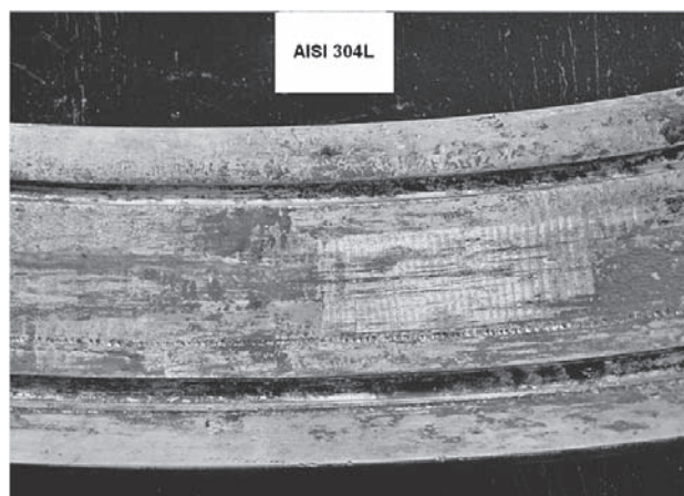
Figure 7 Test semi-ring after use
