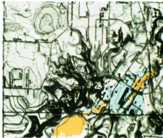
Plate 4. Yellow-colored area shows the effect of specified flood control measures for reducing the extent of flooding from the same storm. Blue shows uncontrolled flood extent, as in Plate 2, for comparison.
