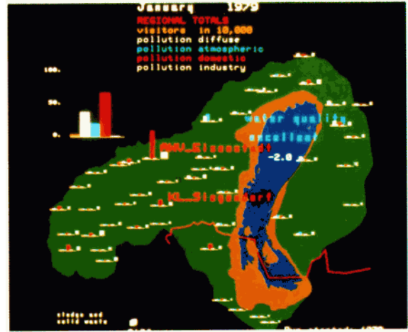
Plate 8. Lake Neusiedl watershed on the Austrian-Hungarian border (red line) showing data from simulation of interaction between tourist and agriculture development and lake water quality.
