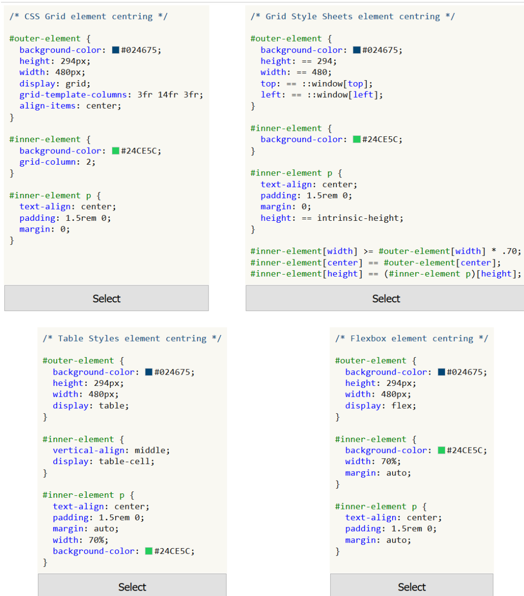
Figure 10: A screenshot of code snippets presented during the experiment. Each snippet accomplishes the same result: positioning a light green element containing text content in the centre of a dark blue element. This is one possible arrangement of the snippets; they are presented in a random order each time the experiment is run. The select button moves the participant to the next step in the experiment.
