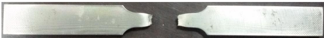
Figure 4.102 A broken specimen of the fatigue test
