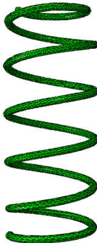
Figure 4.1 Meshing of the coil spring
