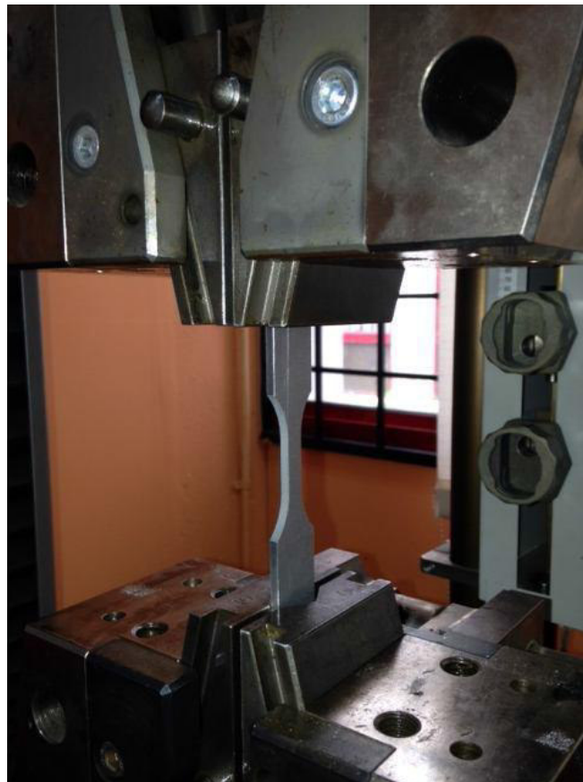
Figure 3.15 A specimen at the Zwick Roell tensile grips
