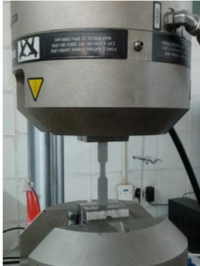
Figure 3.17 A specimen at the Instron fatigue grips
