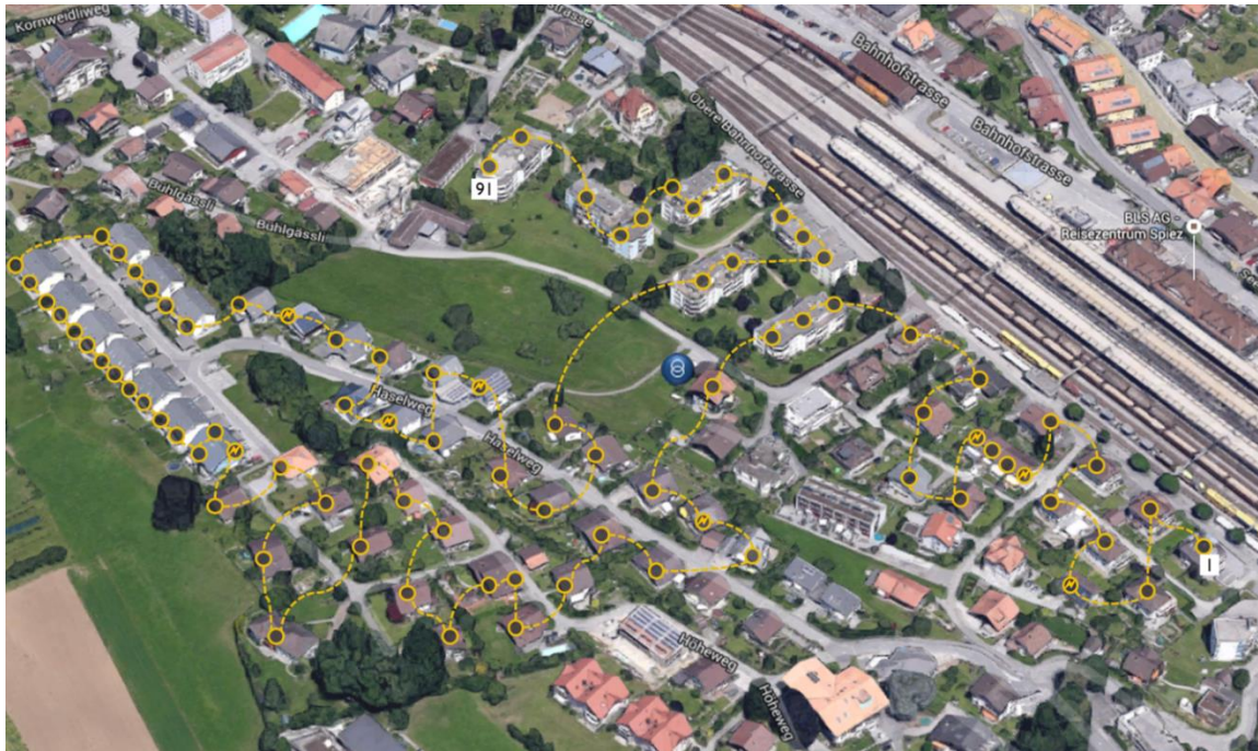
Figure 44: Objects and network structure of transformer station
