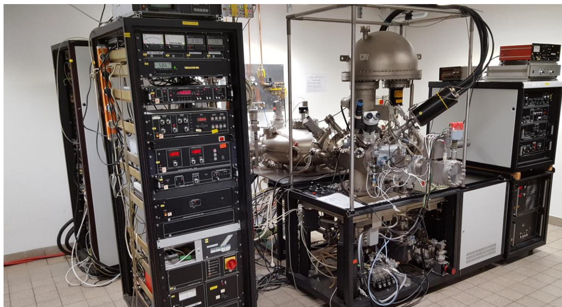
Figure 3.3: A photograph of the XPS setup (MAX 200) used in this PhD work and its components.
