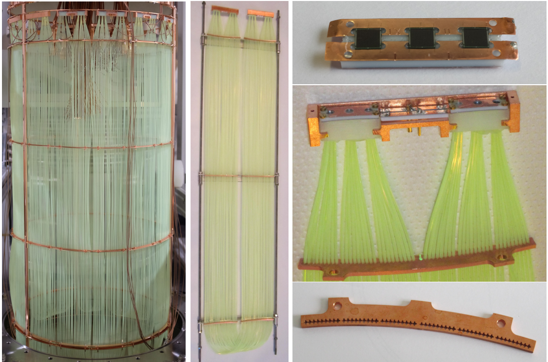
Figure 6.4: Pictures of full fiber shroud and its components. Left) Full fiber shroud. Middle) Two adjoining modules in a mounting frame. Right top) holding frame with three SiPMs. Right middle) top part of a fiber module. Right bottom) copper holder for 54 fibers.
