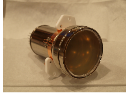
Figure 4.1: Picture of a Hamamatsu Photonics R11065 photomultiplier tube.
