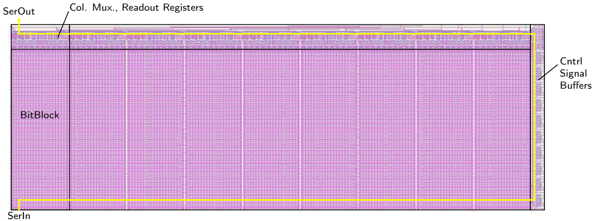
Figure 5.15: Layout of the memory. The memory size is 76 \times 229 \mu\text{m}^2 . The capacity is 800 words of 9 bit, the area of the in-pixel periphery is marginal.
