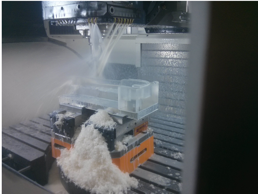
Figure 6.10.: Producing a part of a light-guide using the 5-axis mill at the institute
