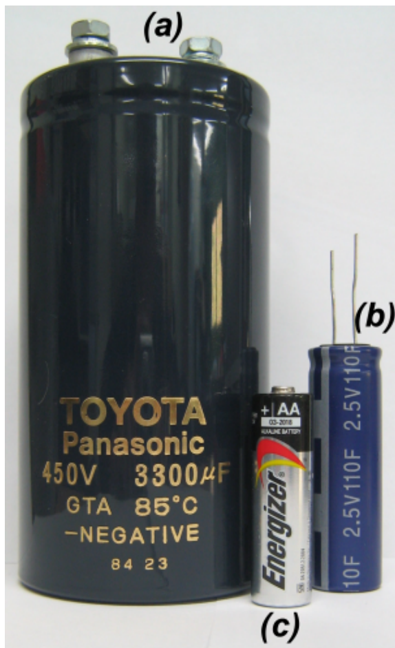
Figure 3.7: Size comparison (a) capacitor from Prius inverter (b) PowerStor Aerogel supercapacitor (c) Energizer AA battery
